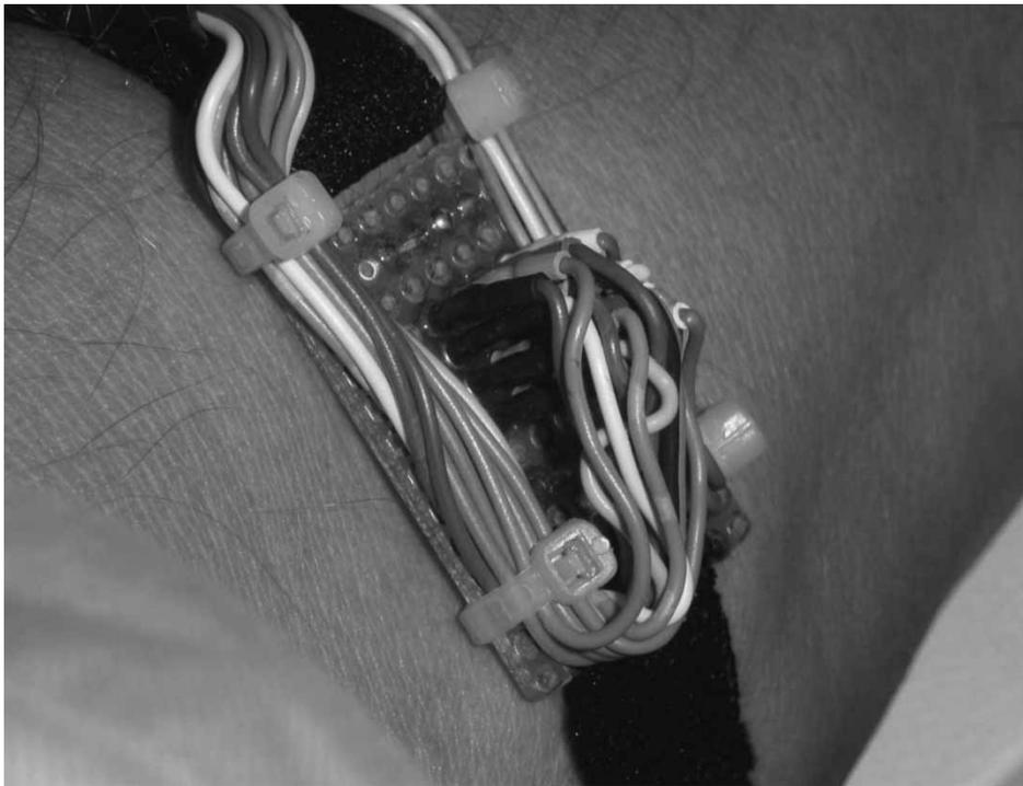
Figure 6. Measurement device for the determination of the electric potential difference. Four times four electrodes serve as sensors and are placed in a distance of 2.4 mm from each other onto the skin surface.
